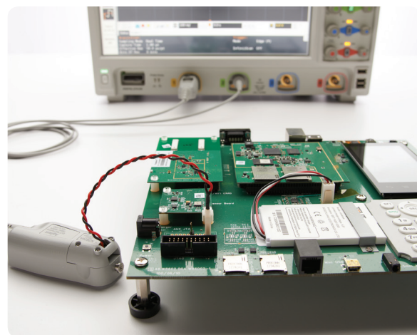
Figure 2. Sense resistor current probe example; Agilent Technologies N2820A
