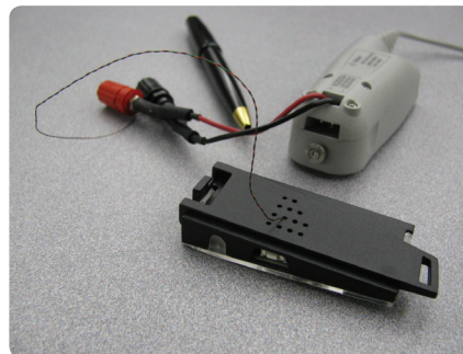
Figure 10. Agilent N2820A current probe connected to measure the current from a mobile wireless device.
